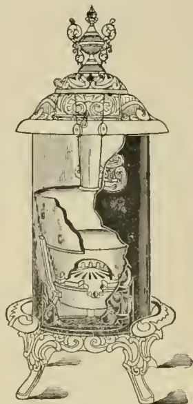
SECTIONAL CUT SHOWING "DOWN-DRAFT."
